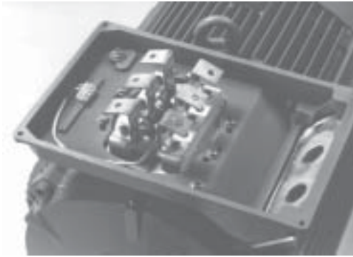
Terminal box of a cast iron motor and of an aluminum motor.
